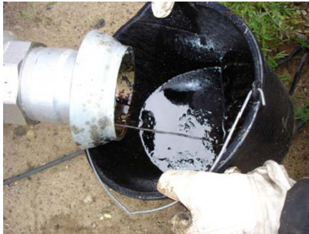
Fig. 10: Separated heavy oil.
