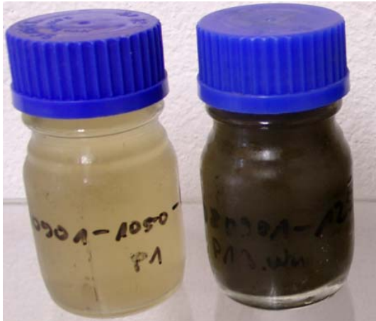
Fig. 7: Transfer of contaminants into the liquid phase (on the left before and on the right after soil washing).
